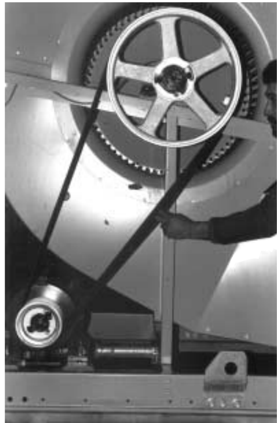
Figure 6 – Fan Belt Adjustment
