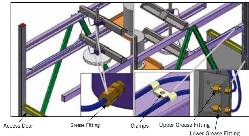
**Figure 3.** Extended Lubrication Lines
