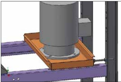
Figure 4. Adjustable Motor Base
