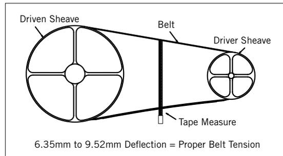
**Figure 5b.** Belt Tension with a Tape Measure
