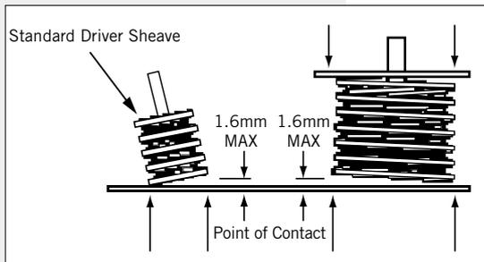
**Figure 6.** Standard Drive Alignment
