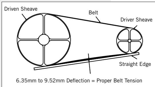
**Figure 5a.** Belt Tension with a Straight Edge
